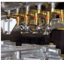
Model 6019SS 1/8 NPT male Material: Type 303 Stainless Steel Max Temp: 400°F (204°C)
